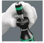
Measurement accuracy is  $\pm$  6 % (article 1430:  $\pm$  10 %) in accordance with the standard DIN EN ISO 6789. Distinctly audible and noticeable excess-load signal when the pre-set torque is reached.
